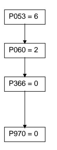
6: Parameter Changes permitted via PMU and Serial Interface (OP1 and PC)
